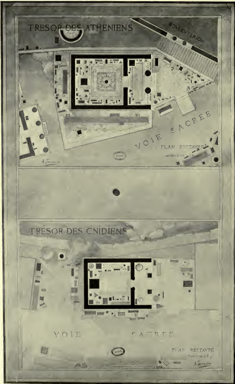
FIG. 19. PLAN OF THE TREASURY OF THE ATHENIANS AT DELPHI. Restored by M. Tournaire.
